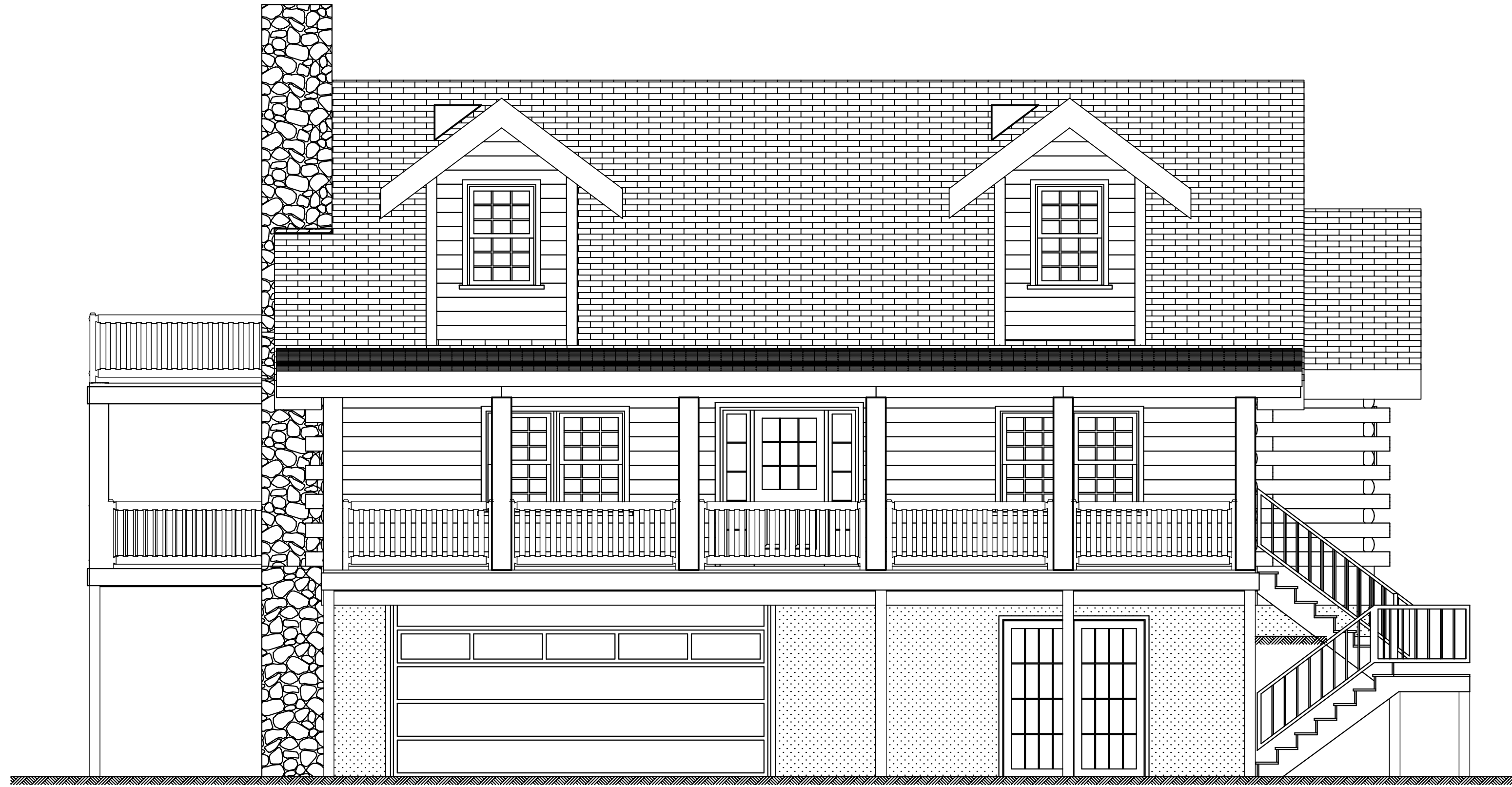
01 Front Elevation SCALE: 1/4" = 1'-0"
